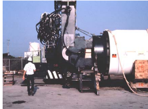
Figure 6. The double-gimbal connection between the CWP and the barge tested off of Honolulu in 1983
